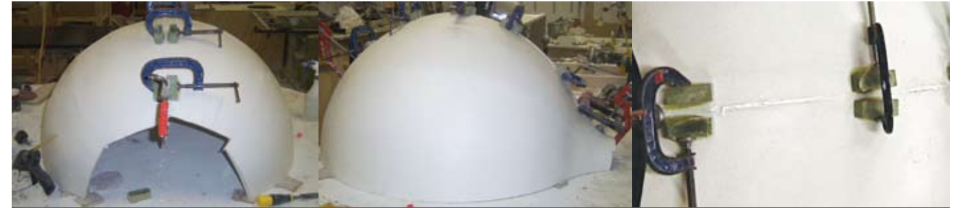
Assembly of 2 quarter pieces to half a shell
